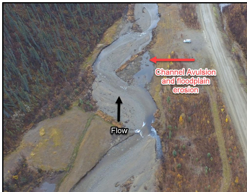
Figure 56. Floodplain erosion and channel avulsion.
