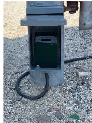
*Pneumatic vehicle counter and housing*
