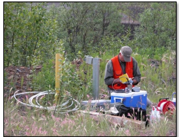
Collecting a groundwater sample from a monitoring well at Red Devil Mine. BLM Photo
