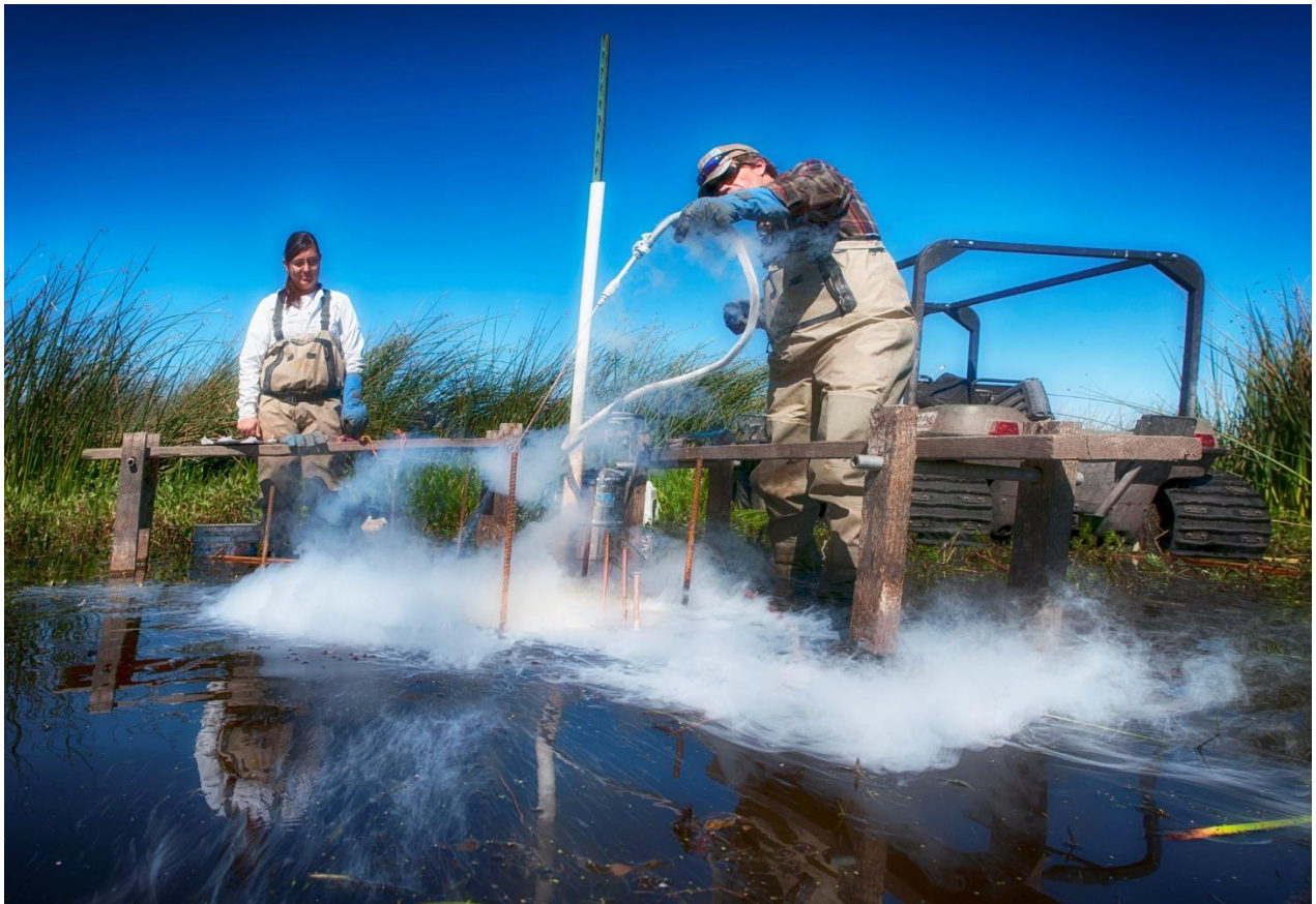
Bureau of Land Management Hydrologist Andy Hamilton and Chelsea Aquino use liquid nitrogen to freeze core soil samples to measure whether wetland restoration actions are having the intended benefit of rebuilding the lost organic soils needed to restore wetland vegetation and functions. Photo by Kevin Abel, BLM. Image taken on 9/19/2013.
